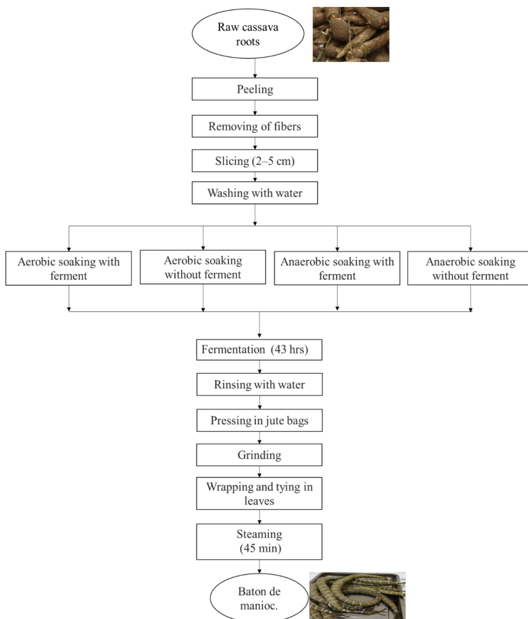
Figure 1. Schematic diagram of Bobolo processing from cassava roots.
